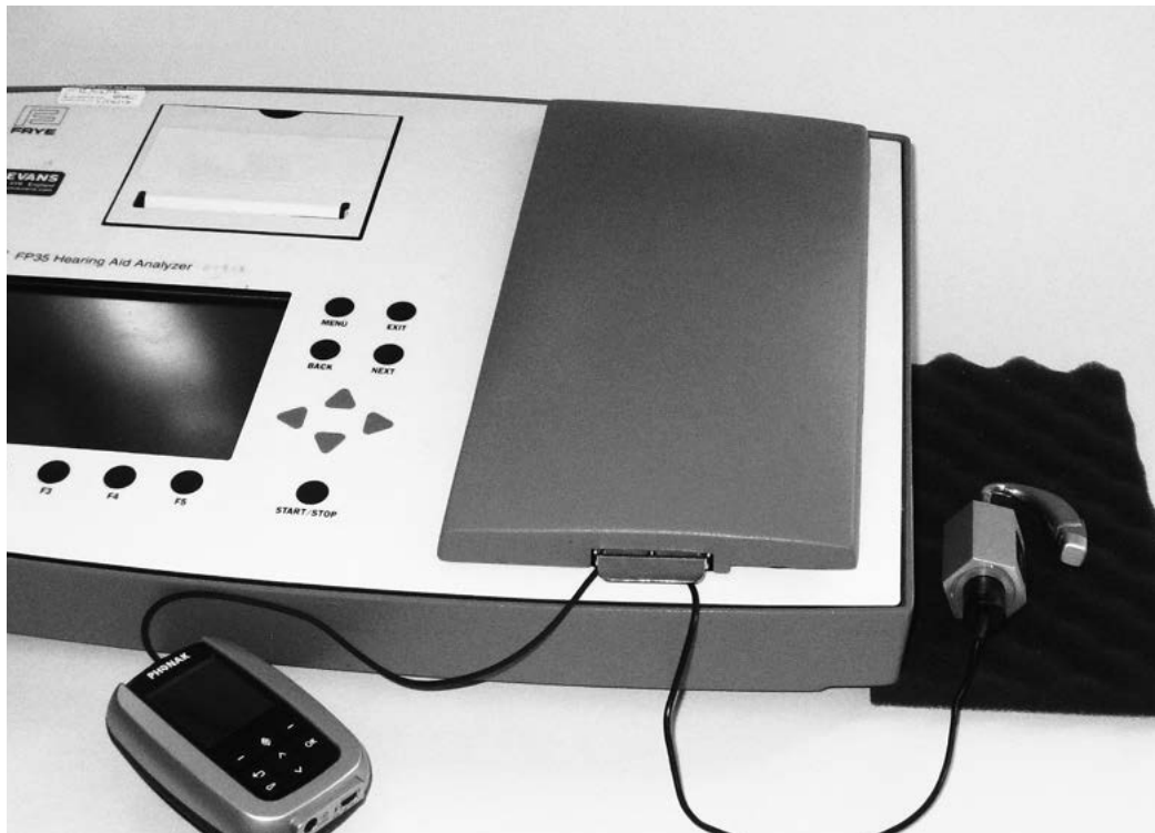
Test box in use for radio aid verification.
